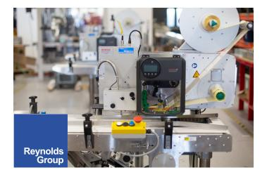
Immediately following, the bottom label is applied through the split-belt to the flat bottom of the tray.
